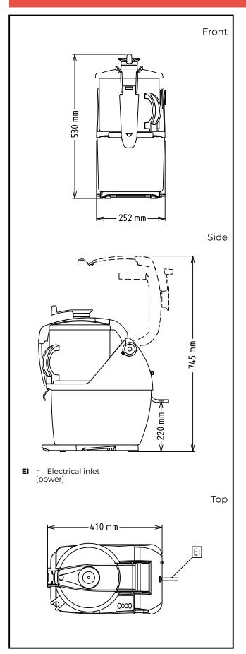
Electric Supply voltage: 200-240 V/1N ph/50/60 Hz Capacity: Performance (up to): 550 kg/hour 7 litres Capacity: Key Information: External dimensions, Width: 252 mm External dimensions, 485 mm Depth: External dimensions, Height: 505 mm **Shipping weight:** ISO 9001; ISO 14001 kg
